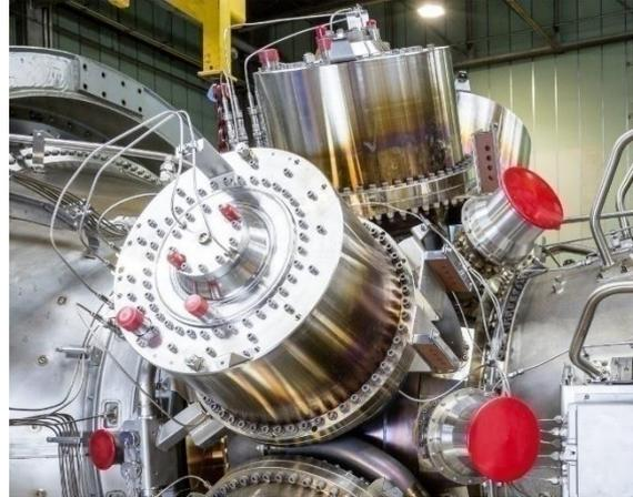
Figure 13: SGT-A65 DLE combustion system
