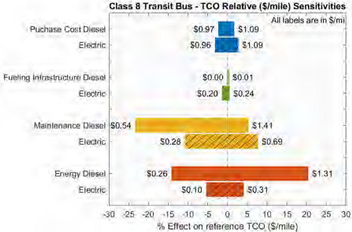
Figure 46: Class 8 Transit Bus TCO sensitivities (listed in Table 23) and their % contribution to reference TCO
