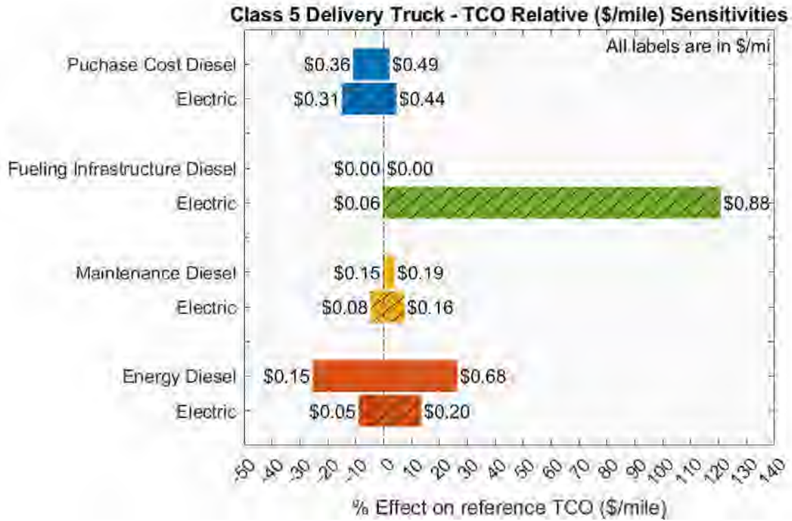
Figure 62: Class 5 Delivery Truck – Sensitivities (listed in Table 30) and their % contribution to reference TCO
