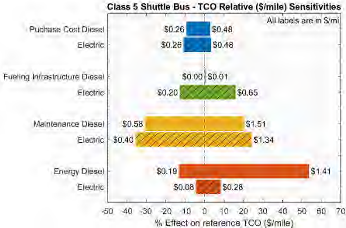
Figure 54: Class 5 shuttle bus – Sensitivities (listed in Table 30) and their % contribution to reference TCO
