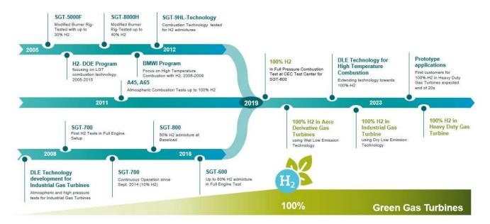
Figure 20: Siemens 100% hydrogen gas turbine roadmap
