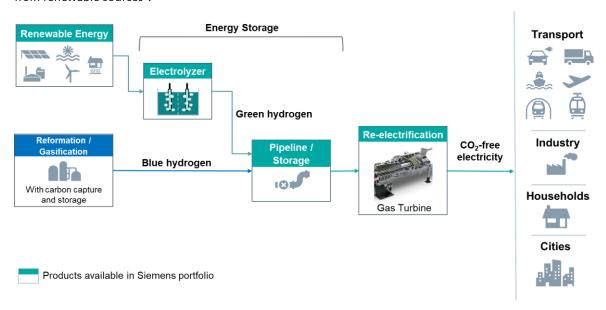
Figure 2: Example of the integration of technologies to produce and use hydrogen
