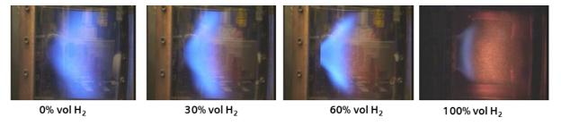
Figure 6: Flame position changes with increasing hydrogen fuel content, showing the most compact flame at 100% hydrogen. Also note how the 100% hydrogen flame is not as luminous as the natural gas flame.
