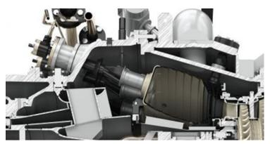
Figure 11: 3rd generation DLE combustion system
