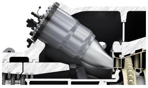
Figure 10: SGT5/6-9000HL combustion system
