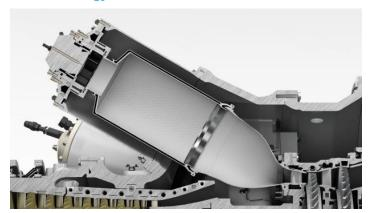
Figure 15: SGT-400 DLE combustion system
