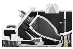
Figure 8: 4000F annular combustion chamber
