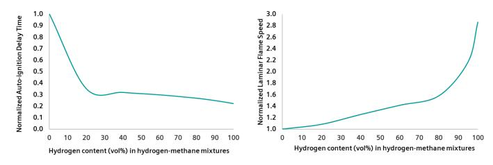
Figure 5: Hydrogen's impact on auto-ignition delay and flame speed for hydrogen-methane mixtures<sup>6</sup>
