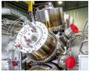
Figure 13: SGT-A65 DLE combustion system
