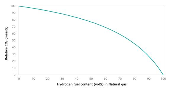
Figure 1: Hydrogen volume percentage (vol%) in the fuel versus the relative CO2 emissions from the combustion process<sup>4</sup>
