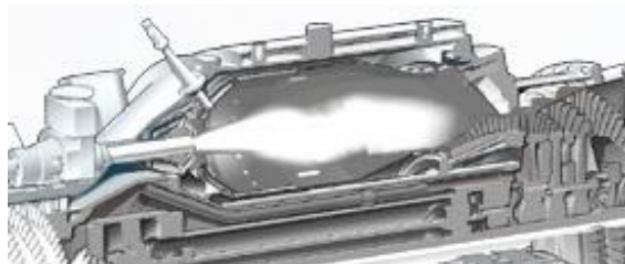
Figure 12: SGT-500 Non-DLE combustion system
