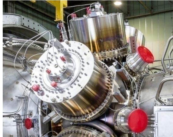
Figure 13: SGT-A65 DLE combustion system
